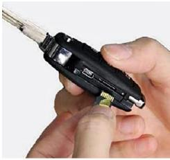
1. Insert the card into the slot like shown in the picture, and please pay attention to the card orientation. Make sure it is inserted properly in the slot before using.
