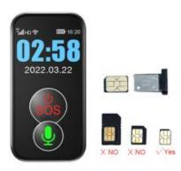
Please turn off the device before inserting the card, as shown in the figure. With the metal side of the card facing up, align the card slot with the upper left corner of the card slot, and then insert the card slot into the device
